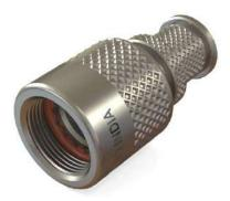
**Free Spinning (3):** Free Spinning Adapters makes the assembly of the backshell to the connector easy without turning the entire backshell body. The coupling nut is free to rotate in this design.
